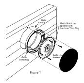
Door Mounting with Grille. If mounting behind factory grilles, omit the trim ring and the grille screen.
